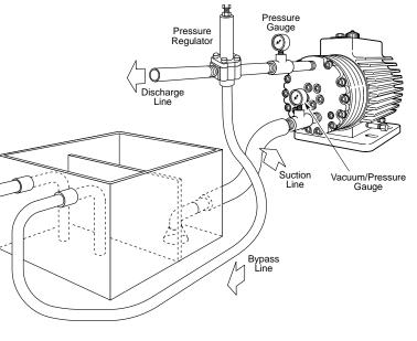
The bypass or outlet lines should be as large as the ports of the regulating valve. Do not install shutoff valves or other restrictions.
