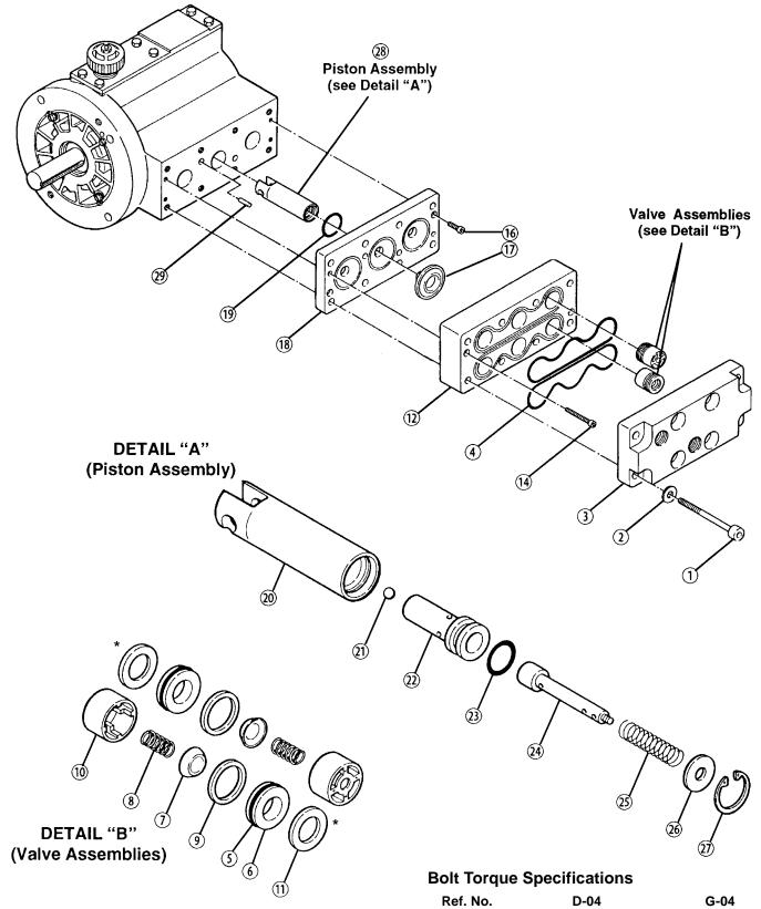
\* Note: dampening washer (11) not used in newer models. The thickness of valve seat (6) is increased on newer models to eliminate the need for the dampening washers.
