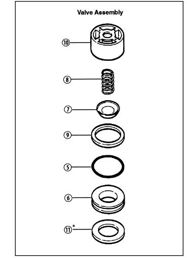
\* Note: dampening washer (11) not used in newer models. The thickness of valve seat (6) is increased on newer models to eliminate the need for the dampening washers.
