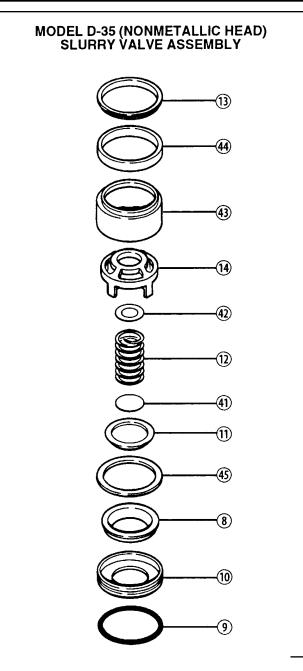
d. Remove the valve seat (8) from its holder (10). Inspect both parts for wear and replace either or both as necessary. It is always a good idea to use a new valve seat and O-ring (9) in the valve seat holder.
