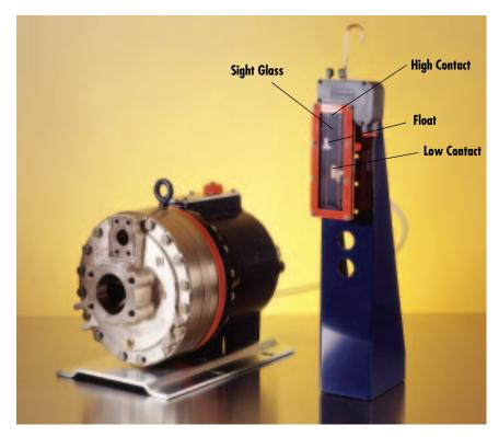
The Hydra-Cell Oil Level Monitoring System utilizes a Murphy SWICHGAGE® Model L129CK1. Field proven in the oil industry to detect crank case oil level, the Murphy SWICHGAGE is well suited to detect oil level for Hydra-Cell pumps such as the D-35 shown here.
