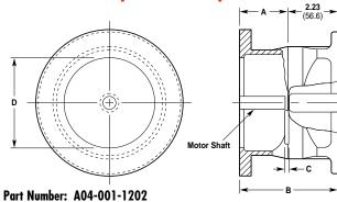
For D-03 and D-04 models for use with 56C, 143TC and 145TC frame motors.
