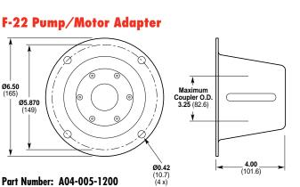
Part Number: A04-005-1200  $\binom{(10.7)}{(4 \times)}$ For F-21 and F-22 models for use with 56C, 143TC and 145TC frame motors.
