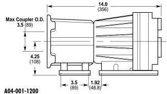
For D-10 models for use with 56C, 143TC and 145TC frame motors.
