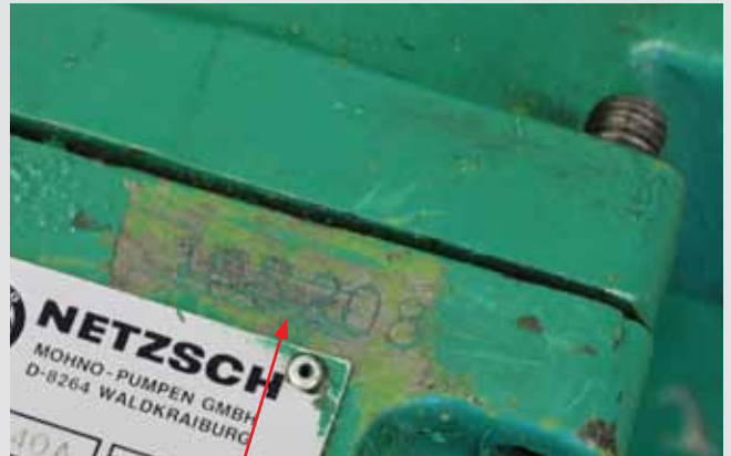
Serial ID number at the top on the bearing housing
