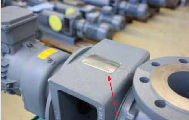
Type plate at the top on the lantern
