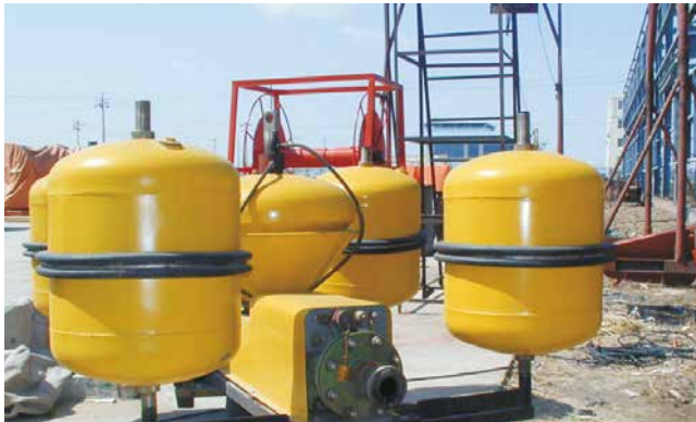
NEMO® pump NM038BY, in floating oil recovering system
