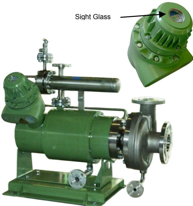
The indicator is visible through a sight glass in the cover of the terminal box. The bright LED's indicate the state of the bearings and the axial position of the rotor. Also a "power on" lamp and indication for correct or reverse rotation are available.
