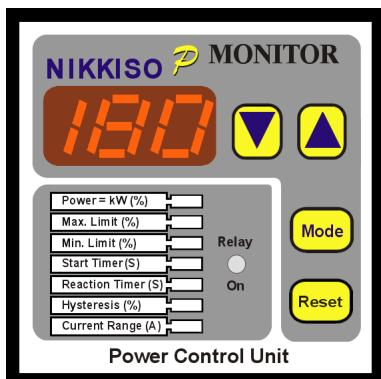
If a pump runs dry, the power consumption decreases. If the quantity of liquid pumped is higher than the design capacity allowed, a max. permissible power consumption can be defined. Both values can be controlled with the Nikkiso P-Monitor and can be used to switch alarms or trip the pump. Operation against closed valve on the discharge side or the min. flow of the pump can also be controlled.
