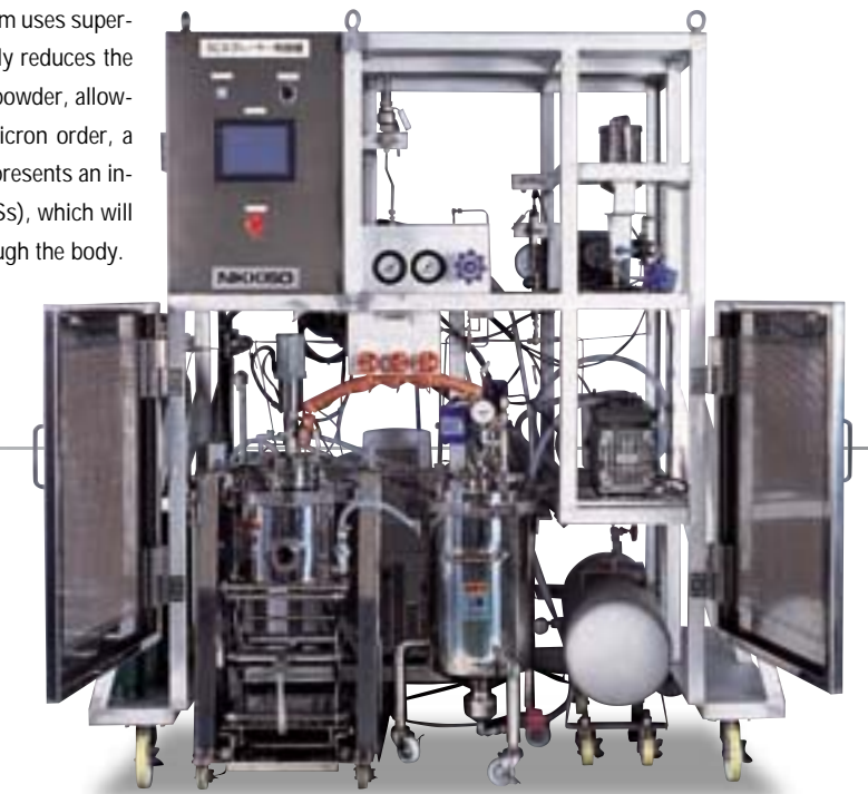
SC-Sprayer( Supercritical ultra-fine powder manufacturing equipment )
