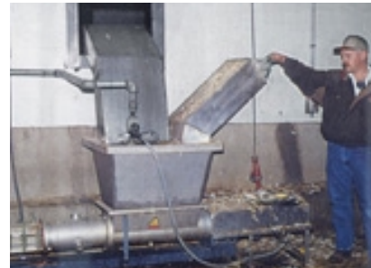
seepex pump BTM 35-6, Product: DOA chickens and chicken waste, Viscosity: <50,000 cPs, Pressure: 3 bar (45 psi), Capacity: 5m 3 /h (22gpm)
