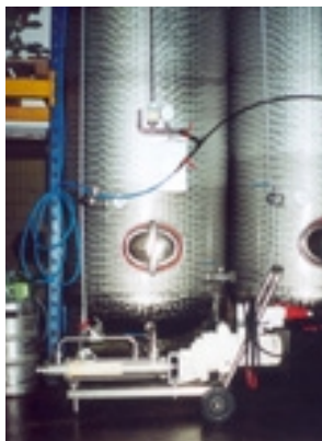
seepex pump BCSB 10-6L, Product: grape mash, Pressure: 2 bar (30 psi), Capacity: 5-7m 3 /h (22-30.8gpm)
