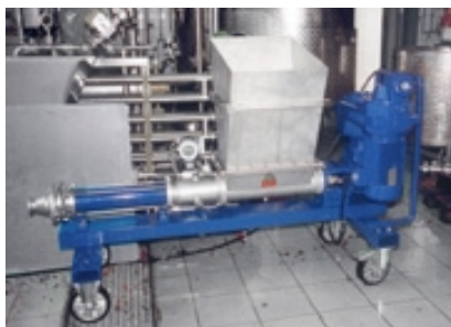
seepex pump BTM 10-12 with stainless steel hopper and mobile cart, Product: cherries, Pressure: 12 bar (175 psi), Capacity: up to 7 m 3 /h (30 gpm)
