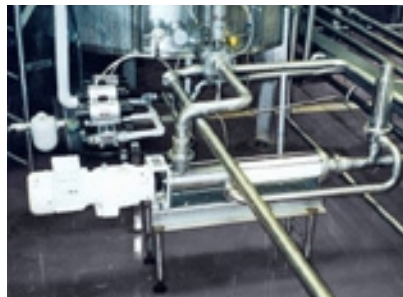
seepex pump BCSB 10-12, Product: diatomaceous earth for filtration, Pressure: 3 bar (45 psi), Temperature: 20-40°C (70-105°F), Capacity: 3m 3 /h (13.2gpm)
