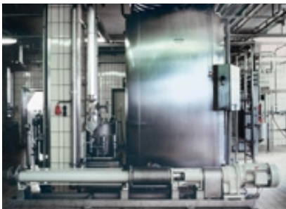
seepex pump NS 35-24, Product: fruit juice, Pressure: 24 bar (350 psi), Temperature: 65°C (150°F), Capacity: 6-13.5m 3 /h (26.4-59.4gpm)
