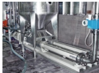
seepex pump BT 35-24 , Product: carrot mash from the degassing tank to the heater, Temperature: 70°C (160°F), Pressure: 20 bar (300 psi), Capacity: 5-10m 3 /h (22-44gpm)
