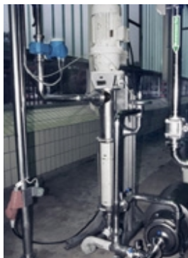
seepex pump BCSO 17-12 , Product: pudding and desserts, Temperature: 25°C (80°F), Pressure: 12 bar (175 psi), CIP cleaning 3% caustic soda and 2% nitric acid at 70-95°C (160-200°F) for about an hour, Capacity: 5-10m 3 /h (22-44gpm)
