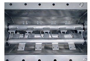
Pump hopper fitted with bridge breaker paddles with teeth for grabbing solid dairy foods such as cream cheese, butter and comparable products.
