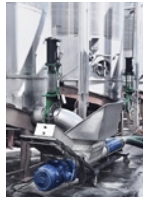
seepex pump BT 130-6L, Product: grape must, Pressure: 3 bar (45 psi), Capacity: 80m 3 /h (352gpm)
