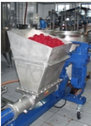
seepex pump BTM 10-12 shredding and simultaneously conveying berries, Capacity: 1-3m 3 /h (4.4-13.2gpm)
