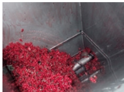
view into hopper of seepex pump BTM 10-12 while shredding and conveying berries
