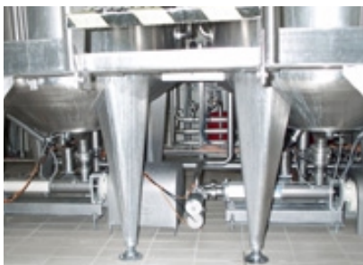
seepex pump BCSO 5-6L, Product: cream cheese with vegetable pieces, Viscosity: 8000 cPs, Temperature: 60°C (140°F), Pressure: 4 bar (60 psi), CIP cleaning: at 80°C (175°F) with 2% NaOH solution, at 65°C (150°F) with 1% HNO 3 solution, Capacity: 0.1-1.5m 3 /h (0.44-6.6gpm)
