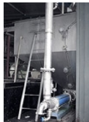
seepex pump BTM 70-12 for chopping and simultaneous transporting of apples, Pressure: 6-12 bar (90-175 psi), Temperature: 20-30°C (70-90°F), Capacity: 15-20m 3 /h
