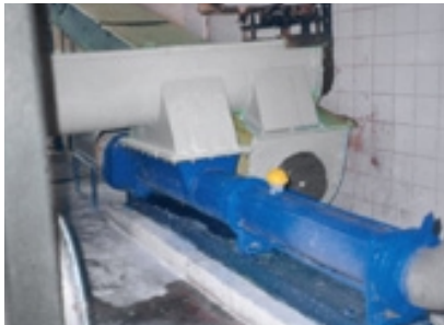
seepex pump BT 70-6L, Product: fish concentrate, conveyed into separator, Temperature: 90°C (195°F), Pressure: 2 bar (30 psi), Capacity: 12-22m 3 /h (52.8-96.8gpm)
