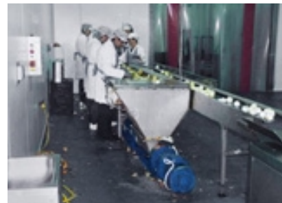
seepex pump BTM 17-12 and inspection conveyor belt
