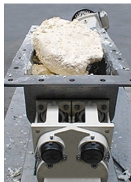
seepex pump BTCI 10-12 for mashing and conveying soft cheese, Viscosity: non flowable, Temperature: -1.3-2.0°C (30-35°F), Pressure: 7 bar (105 psi), Capacity: 2,3m 3 /h (10.12gpm)
