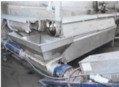
seepex pump BT 130-6L, Product: grape must, Pressure: 4 bar (60 psi), Capacity: 75m 3 /h (330gpm)
