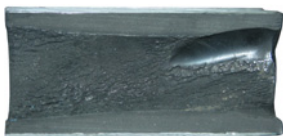
non-original damaged stator
