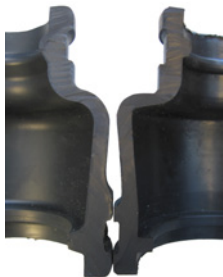
seepex original joint sleeve vs. non-original joint sleeve
