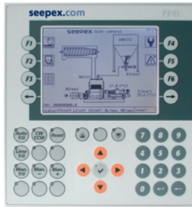
Control device with various display pages permits simple and user-friendly operation
