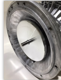
Curve of center disk to face out.
