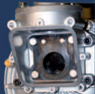
Only 4 bolts to access flap valves
