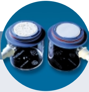
Spallation debris collected onto a microporous filter membrane after recirculating water for 48 hours through thermoplastic elastomer tubing (left) and STA-PURE tube (right). The thermoplastic elastomer tube produced particles of rubber, inorganic filler, and plasticiser.
