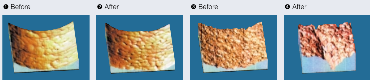
Profilometric scan of STA-PURE tube (1 and 2) compared to thermoplastic elastomer tube (3 and 4), before and after pumping.
