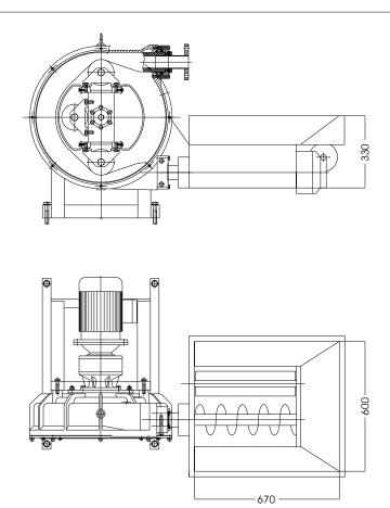
The feed hopper is an accessory which is available for our model FMP-60, and consists of a hopper holding an endless feed screw, a second turbulence break-up vane, together with its own geared motor. The complete assembly is manufactured in stainless steel.
