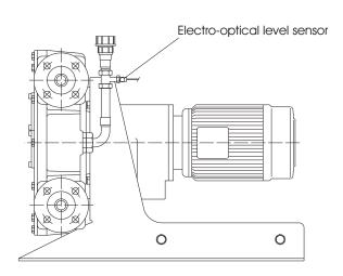
Due to its construction characteristics, the peristaltic pump has practically only one wearing element, that is the tube.
