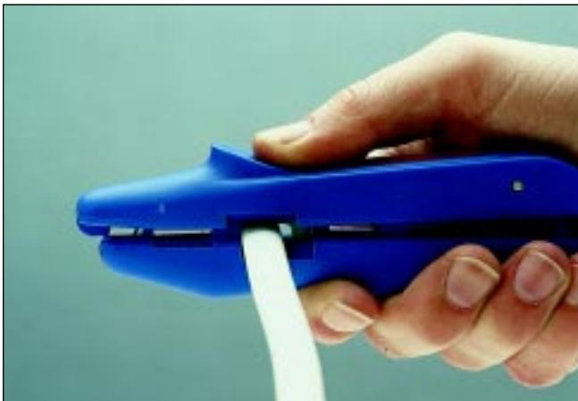
For cable and wire stripping of flat cables with only one tool.
