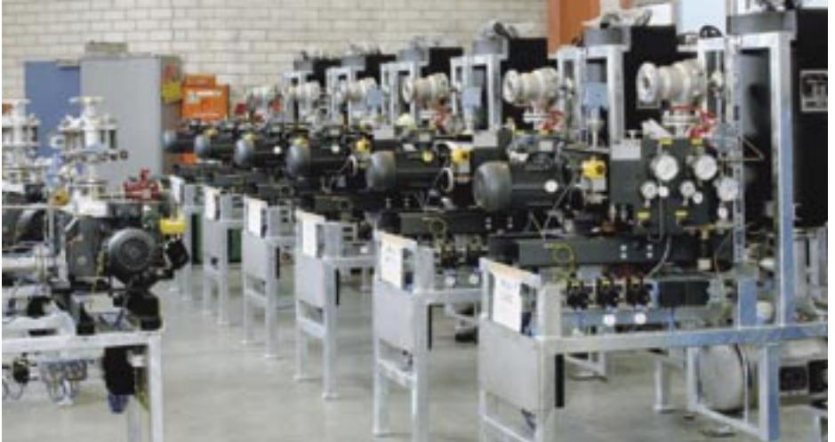
Screw vacuum pumps, category 1(i) devices in accordance with directive 94/9/EC for the pharmaceutical industry
