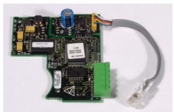
Each fieldbus interface for the Commander SE is a single option card that fits within the drive. Parameter data is transferred to and from the Commander SE using a 2-wire RS485 link into the serial communications port on the drive.
