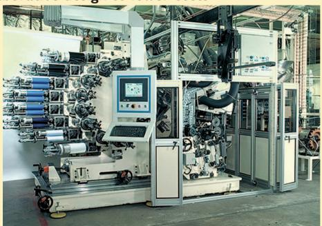
This oval-tube packaging printer has over 40 servomotors and several AC induction motors. Cost savings were achieved using the Unidrive 🔊 with an SM-Applications module together with several Commander SE drives to complete this one-of-a-kind machine.
