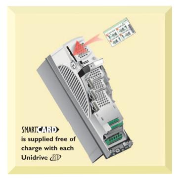
The drive only communicates with the **SMART(4.171)** when commanded to read or write, meaning the card may be "hot swapped".
