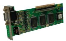
One Daughter Board will control up to 3 axes with each having an independent ( channel to achieve the high speed update of 125 µS. Up to 12 (channel to achieve may be used in an MC control system.
