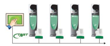
Some Horner products are able to connect directly to Control Techniques drive-to-drive network CTNet by fitting an optional network adapter to the operator interface.
