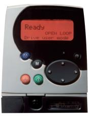
SM-Keypad Plus, designed for use with Unidrive IP and Commander SK, has a multi-lingual backlit LCD display with three lines of text. Line I shows drive status or current menu and parameter number plus parameter value or the specific trip. Lines 2 and 3 show the parameter name or the help text.
