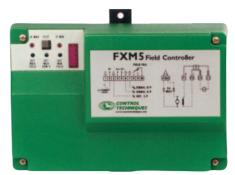
The FXM5 field regulator is designed to control the field current of DC motors up to 20 amps. When used with the Mentor II variable speed DC drives, the field regulator is controlled directly via the drive parameters. This allows full customization of the field control for any application. The FXM5 can also be used as a stand-alone unit when retrofitting existing applications.
