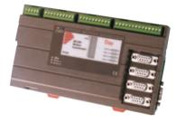
Equipped as standard with a single axis and a reference encoder, the MC206 may be fitted with a Trio (Sig) Daughter Board to provide 3 further axes
