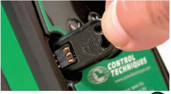
The drive only communicates with the SmartStick when commanded to read or write, meaning that it may be "hot swapped".
