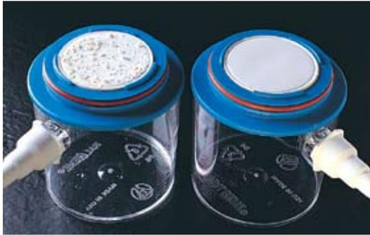
Spallation debris collected onto a microporous filter membrane after recirculating water for 48 hours through thermoplastic elastomer tubing (left) and GORE® High-Resilience Tubing Style 100 (right). The thermoplastic elastomer tubing produced particles of rubber, inorganic filler and plasticizer. There was no shedding from the GORE® High-Resilience Tubing Style 100.
