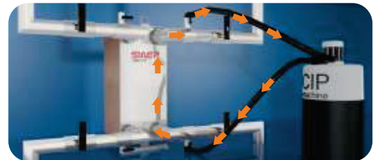
Connect the CIP machine via inlet/outlets on front or back. Pump the solution into the BPHE using the lower connection to expel air. Reverse the flow direction every 30 minutes.
